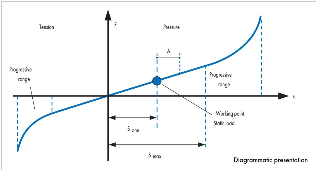
Fig. 8 Working point and oscillation amplitude
