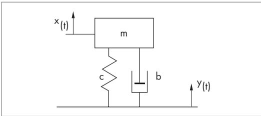
Fig. 2 Single-mass oscillator
