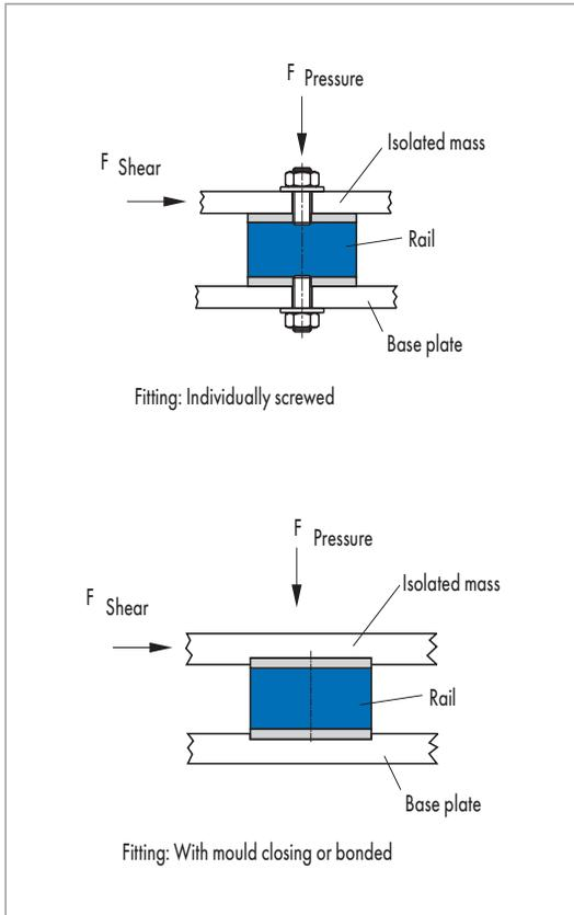
Fitting & installation: rails with load directions
