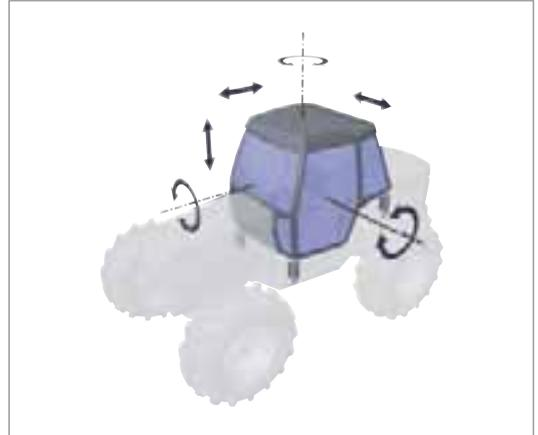
Fig. 4 Movement possibilities of the cabin
