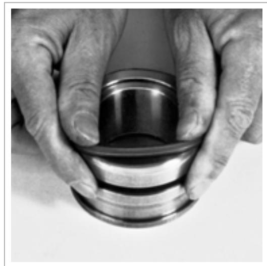
Fig. 44 Snapping in the polyurethane running ring
