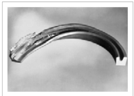
Fig. 18 U-ring destroyed by hydrodynamic pressure build-up
