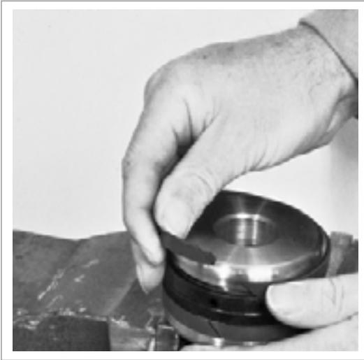
Fig. 49 Snapping in the guide back-up ring
